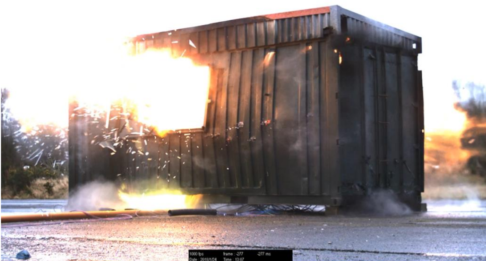
Figure 38: Burning gases venting from windows (approx. time after ignition - 110 ms)
