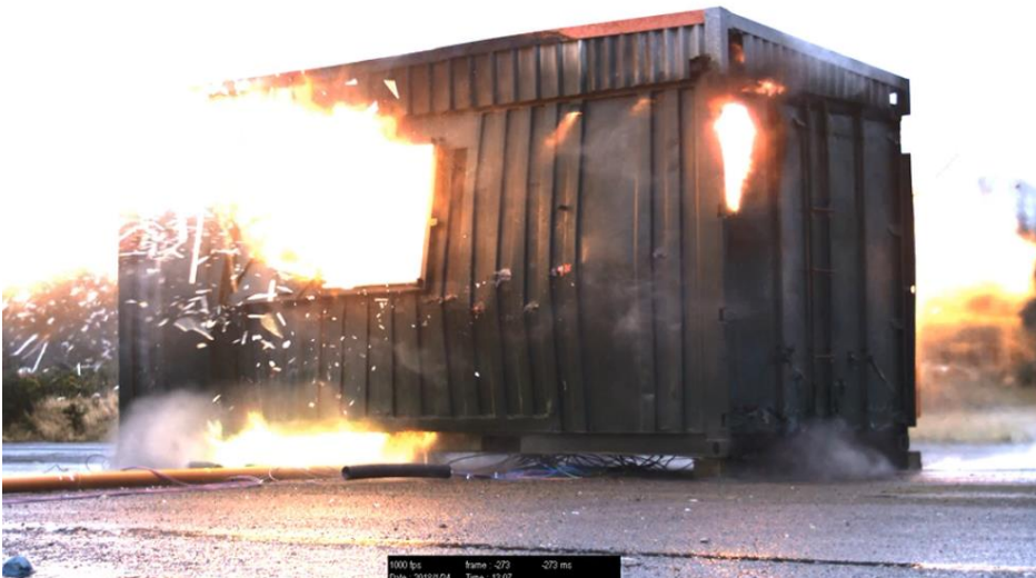
Figure 40: Burning gases venting through windows, bottom and sides of container (approx. time after ignition - 150 ms)
