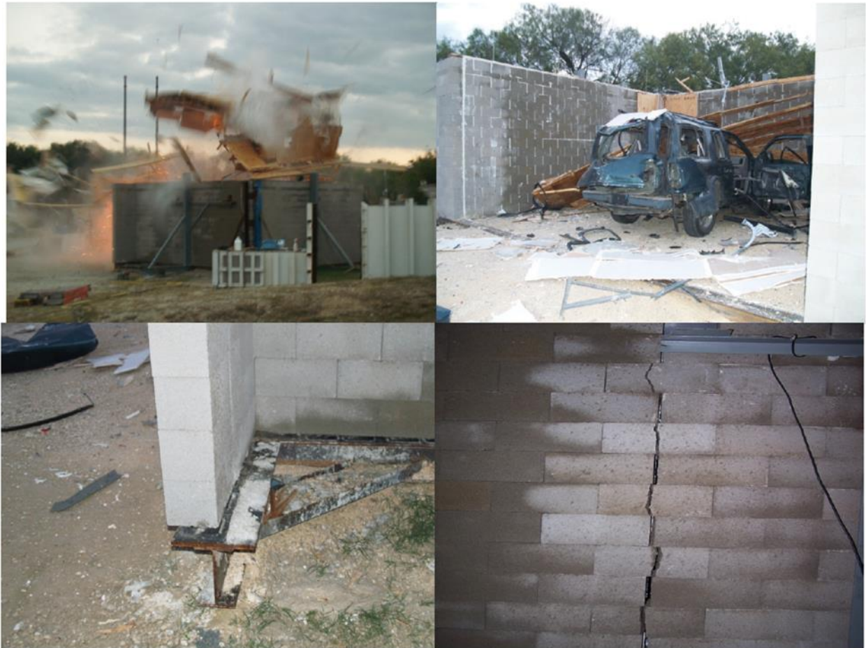
Figure 7: Blast damage from the 17.7% test with vehicle [14]
