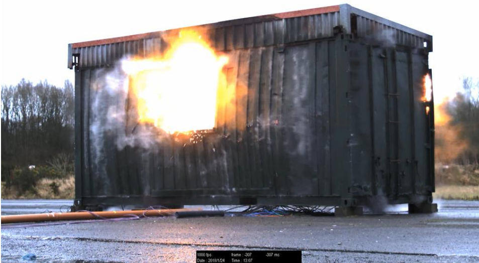
Figure 38: Burning gases venting from windows (approx. time after ignition - 110 ms)
