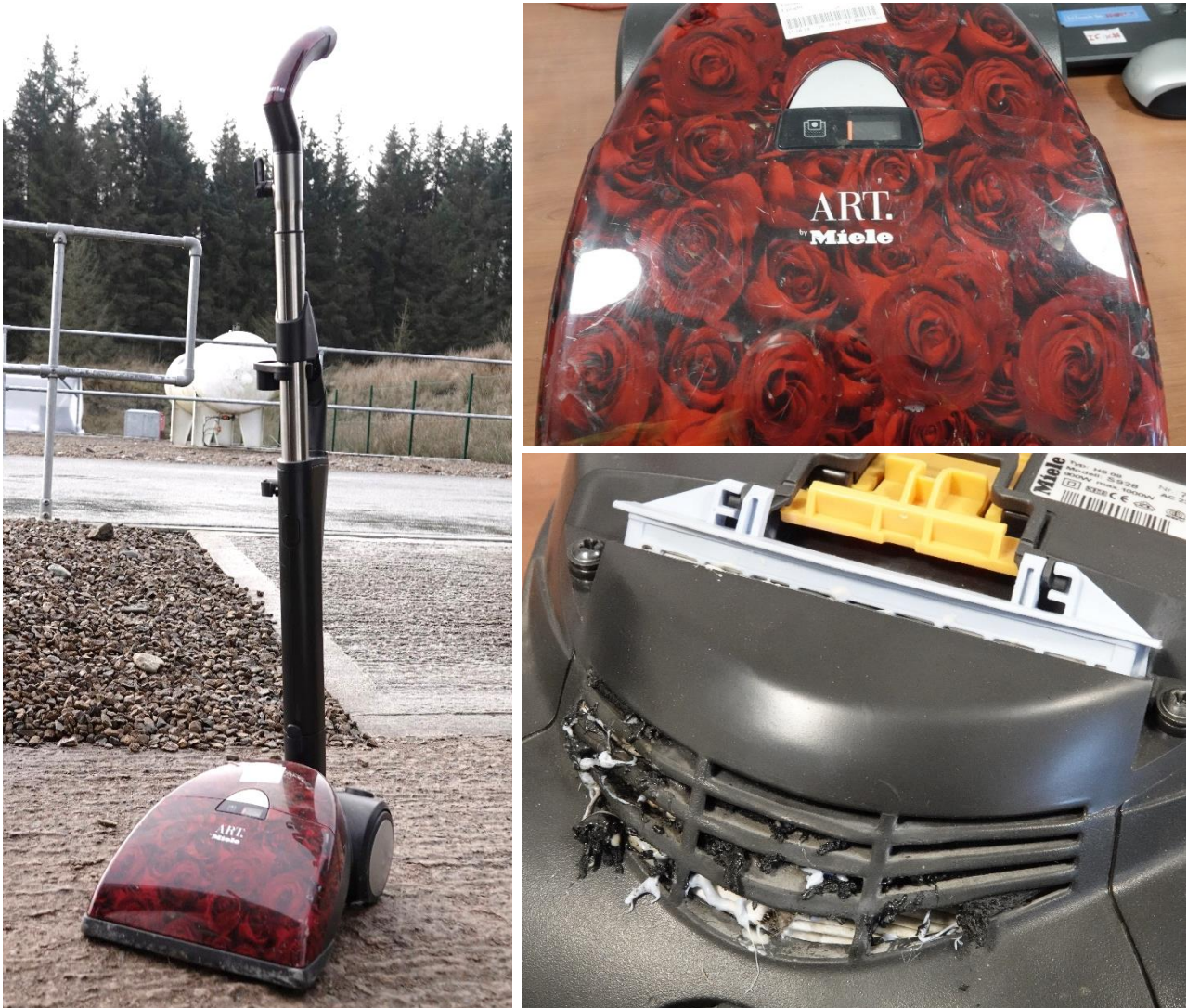
Figure A.14 – Old vacuum cleaner. Left: as tested state., Upper right: front of casing. Bottom right: filter slot showing melting and expansion damage.
