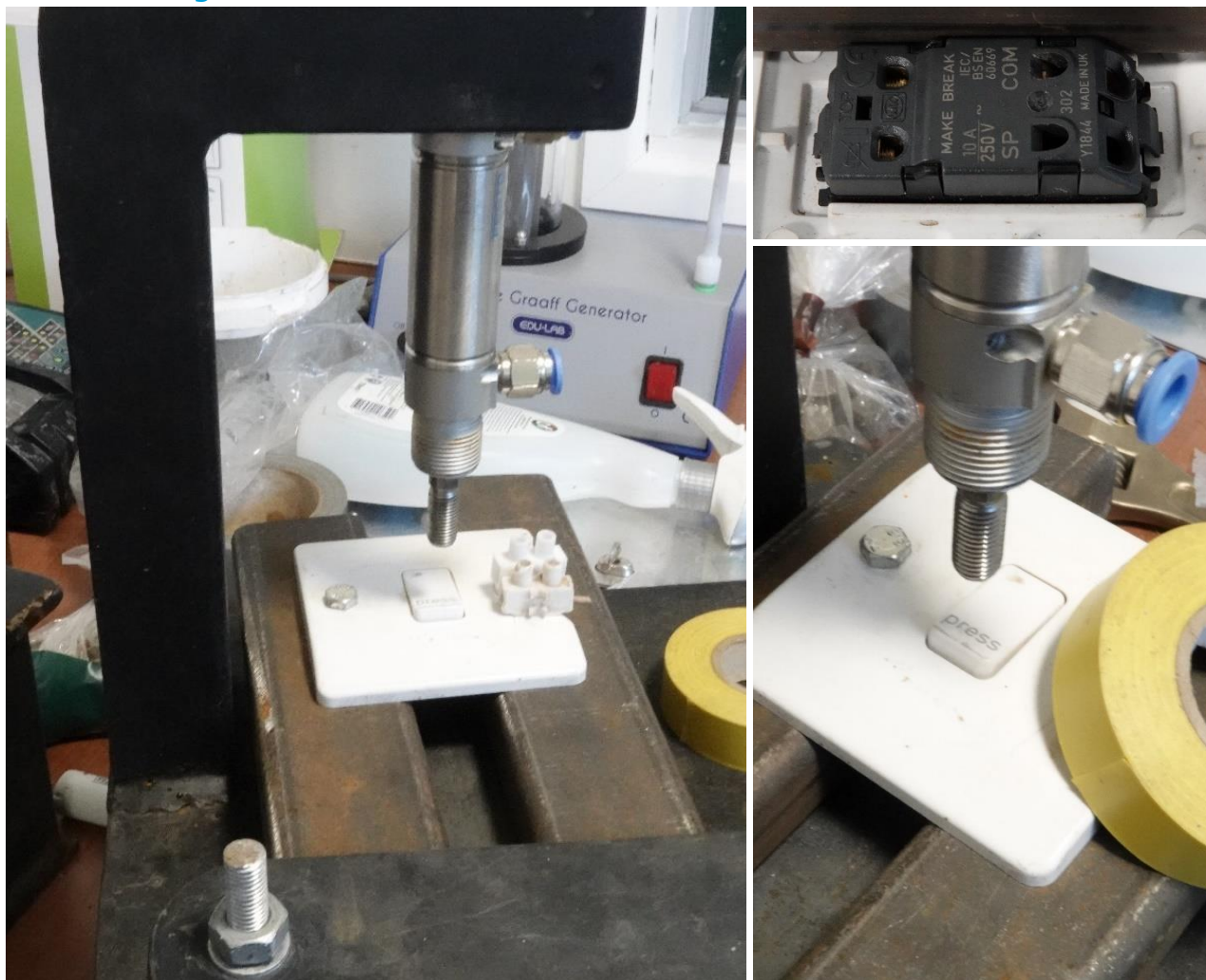
Figure A.2 – Push light switch. Left: switch installed underneath a pneumatic ram. Upper right: connections on reverse side of switch. Lower right: closeup of ram over switch.
