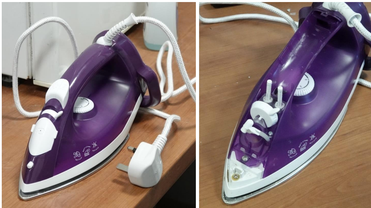
Figure A.18 – Tesco’s Iron. Left: before testing. Right: after explosion in hydrogen, top part of housing has been blown away
