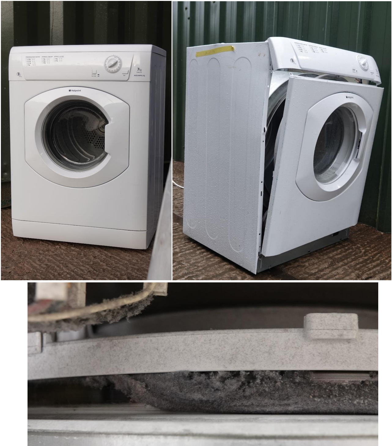
Figure A.16 – Hotpoint Aquarius TVM570. Upper left: as tested state. Upper right: after hydrogen explosion, Lower: separation of drum (upper) from chassis (lower).
