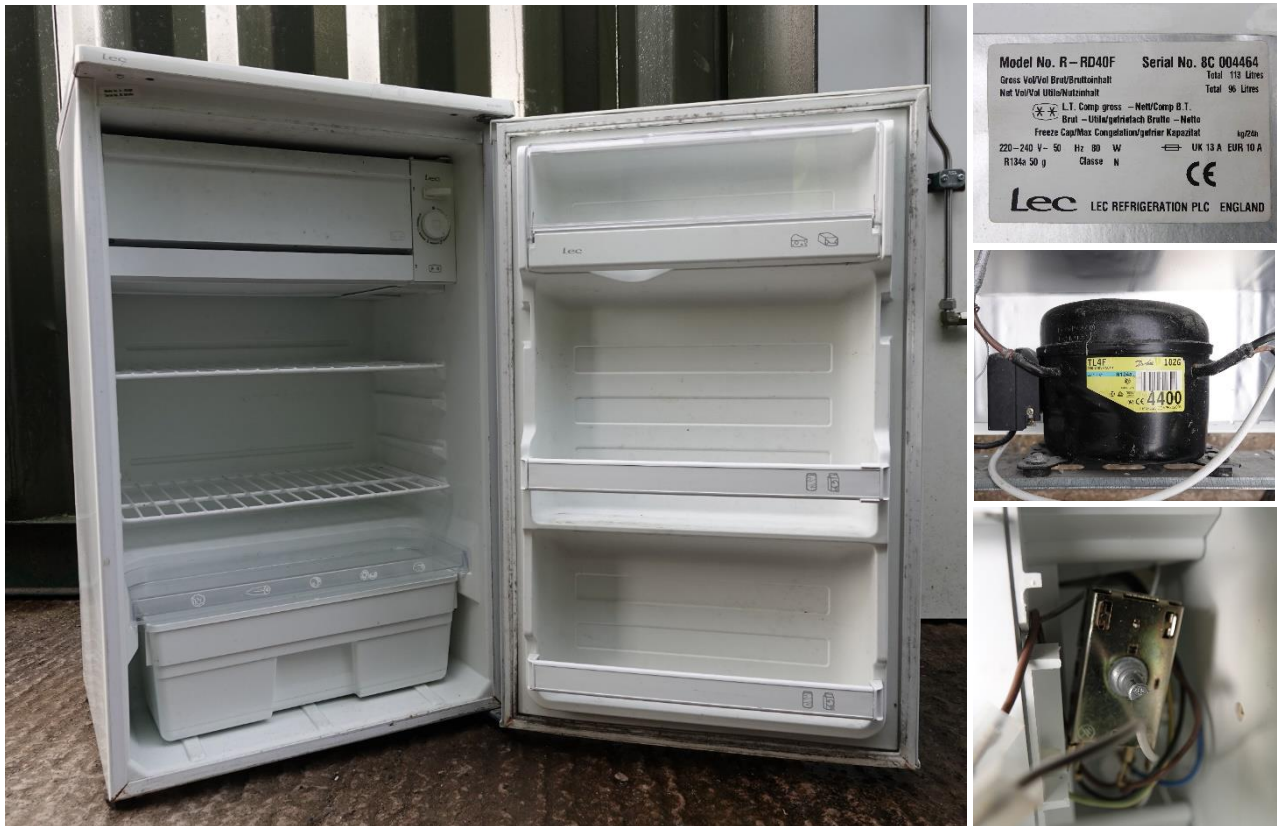
Figure A.17 – LEC R-RD40F Fridge unit. Left: as bought condition showing unmodified control unit internally (main body top-right). Upper right: label. Central right: compressor unit. Lower right: switching mechanism.
