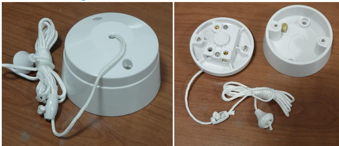
Figure A.3 – Pull cord light switch. Left: switch before tests. Right: underneath of switch with base removed.
