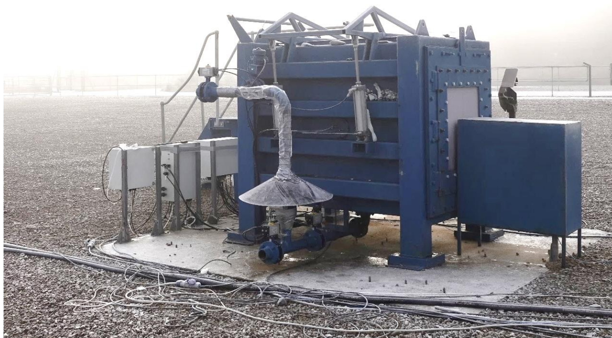
Figure 1 - Explosion chamber used for ignition potential experiments
