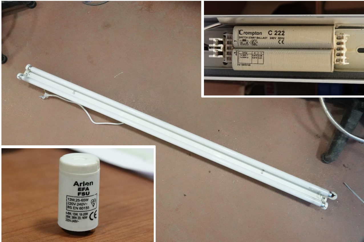
Figure A.12 – Fluorescent light fitting. Centre: entire fitting. Lower left: ignitor
