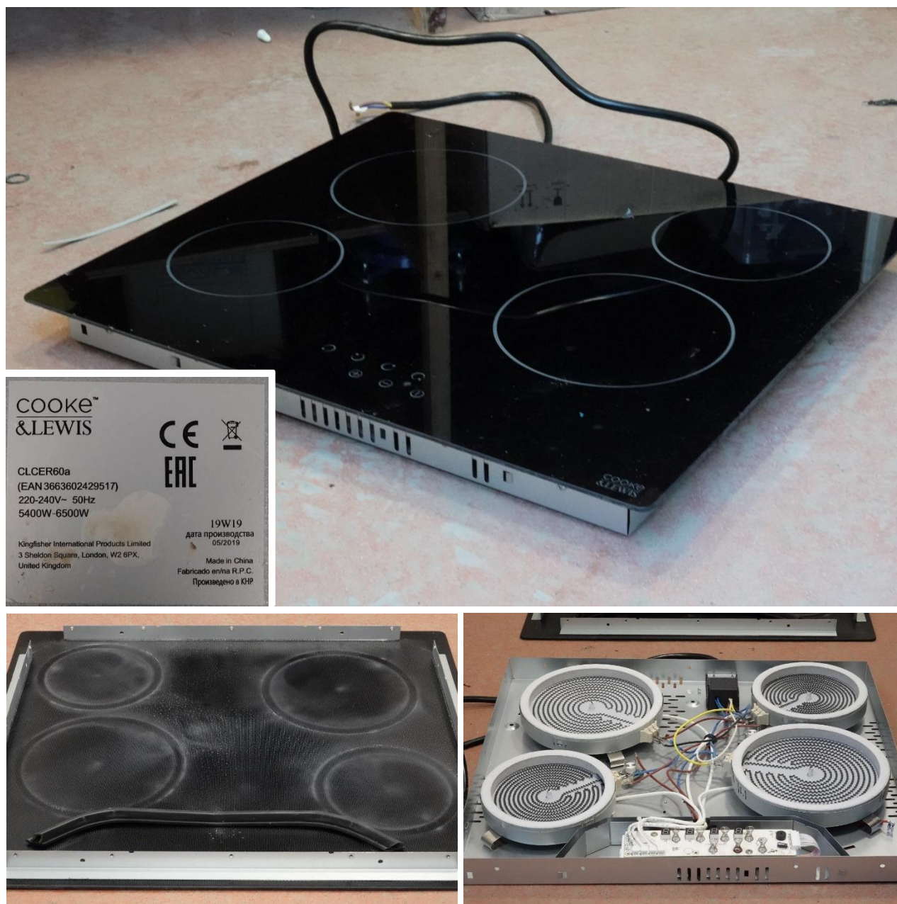
Figure A.20 – Cooke & Lewis CLCER60A Electric Hob. Upper: as tested condition., Middle right: label., Lower right: exposed heating elements., Lower Left: inside of glass top after testing.
