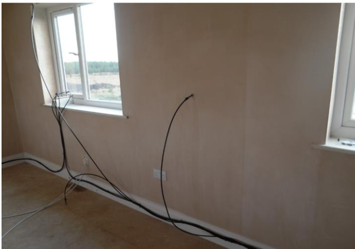
Figure 26: Cavity wall sample point on 1 st floor
