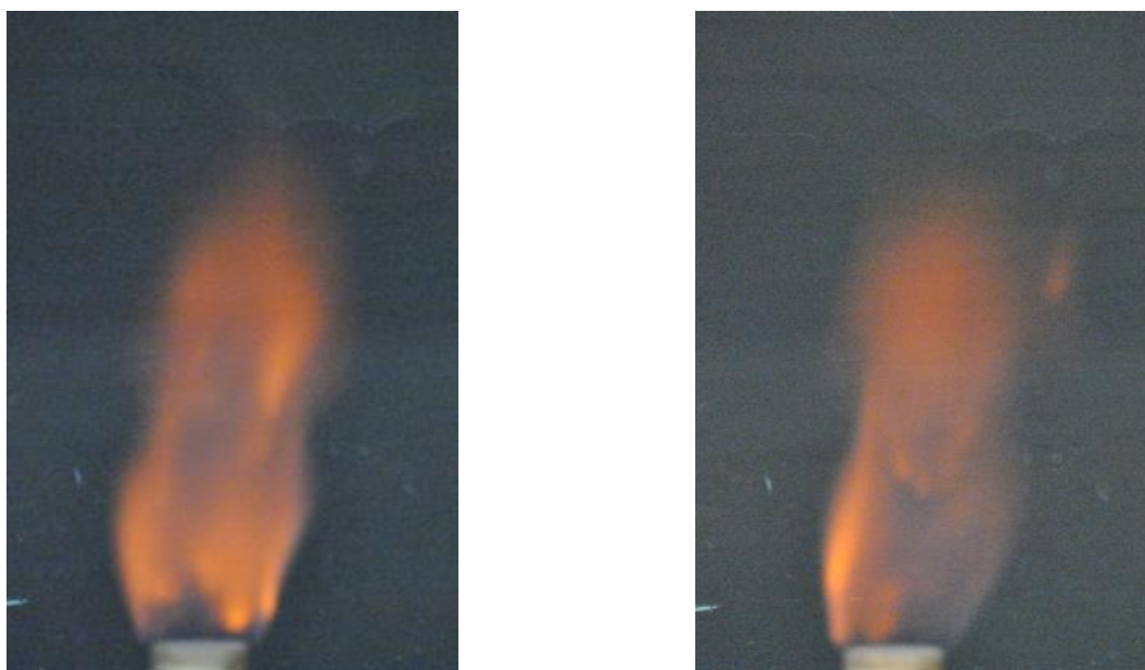
Figure 16: Comparison of hydrogen flames (unodourised - left-hand side; odourised - right-hand side)
