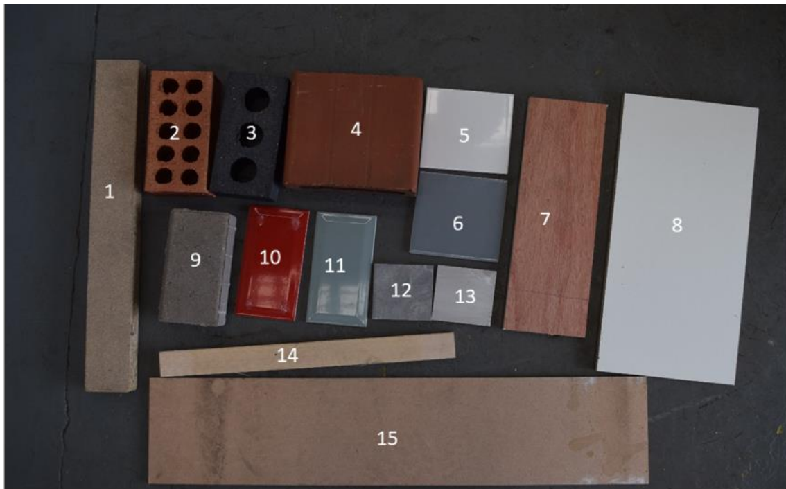
Figure 17 - Selection of background materials used for the flame visualisation studies
