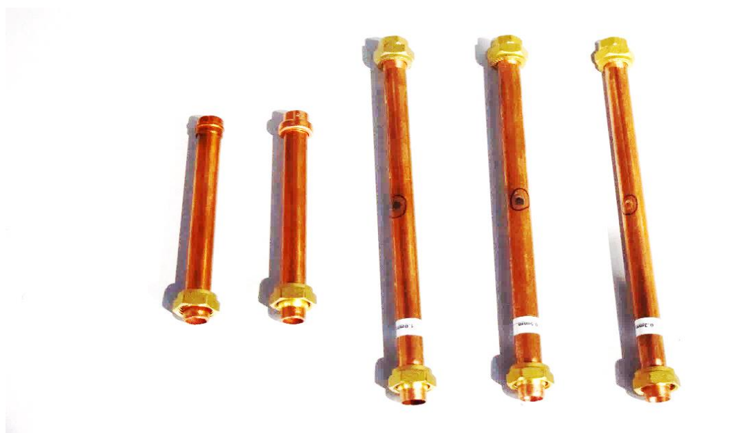
Figure 23 - Copper pipe test pieces (from left to right) - unsoldered end cap, "push-fit" end cap, 0.3mm (left), 0.5mm (middle), 1.0mm (right)
