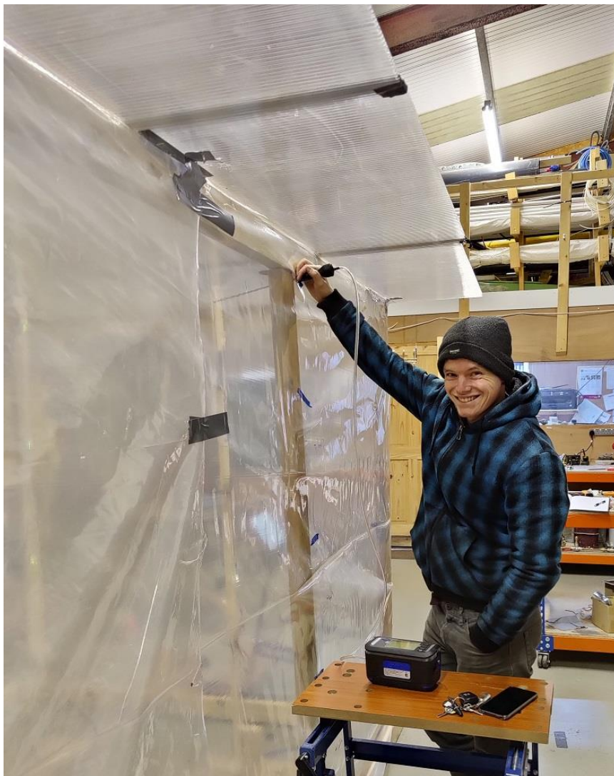
Figure 70: Taking hydrogen readings from the GMI GS700H
