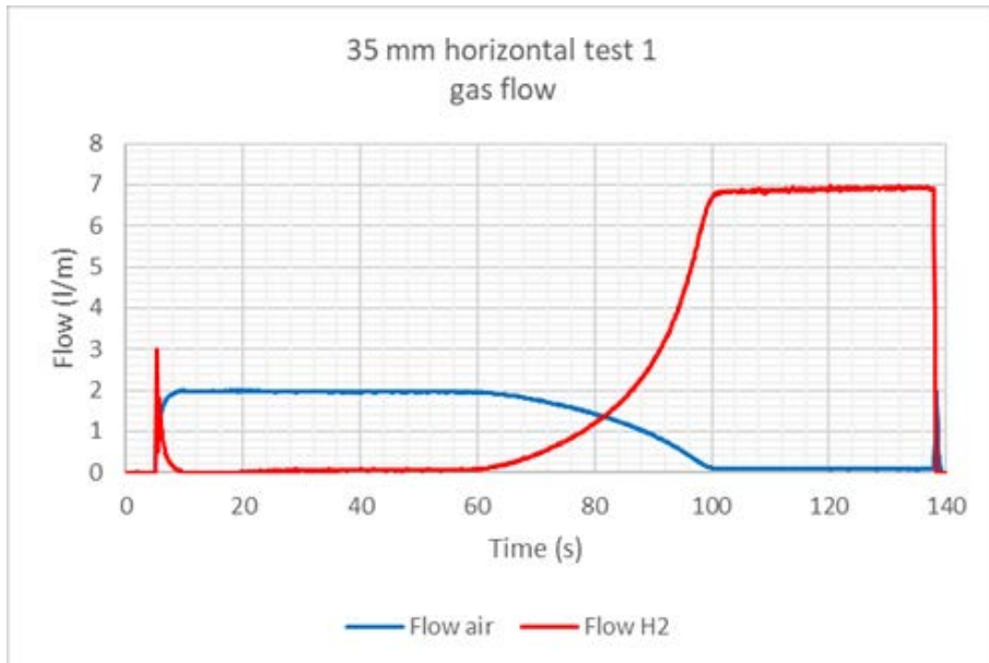
Figure 16: Result graph #3, calculated air and hydrogen flow out of the purge point
