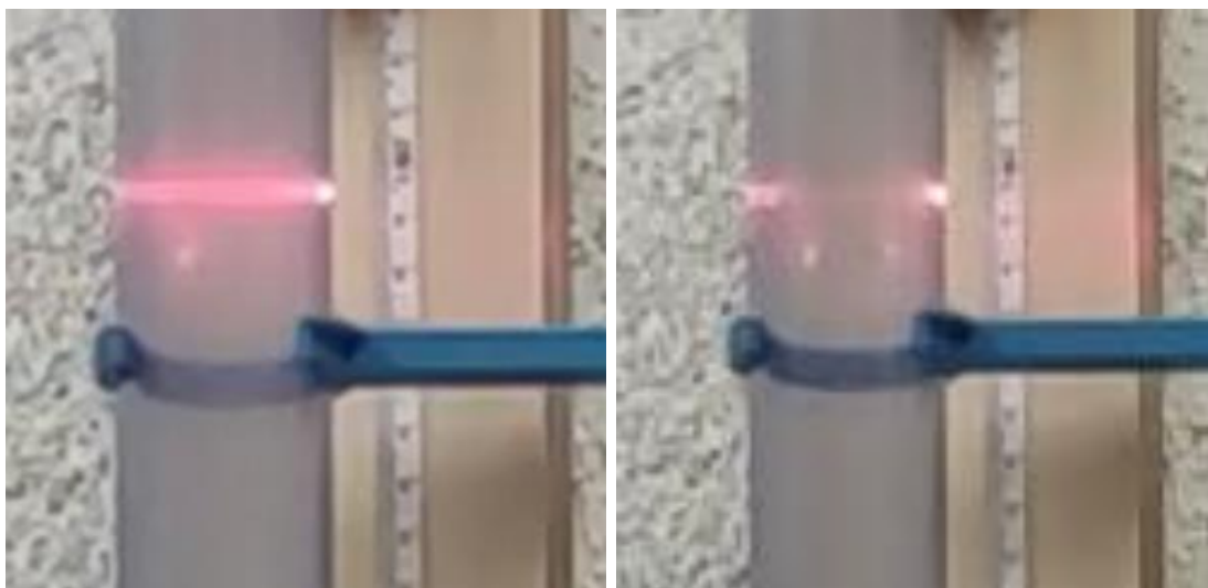
Figure 8: Laser markers indicating vapour (LHS) and no vapour (RHS)
