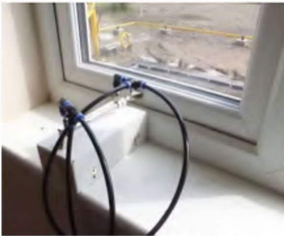
Figure 14: Pneumatically operated window ram
