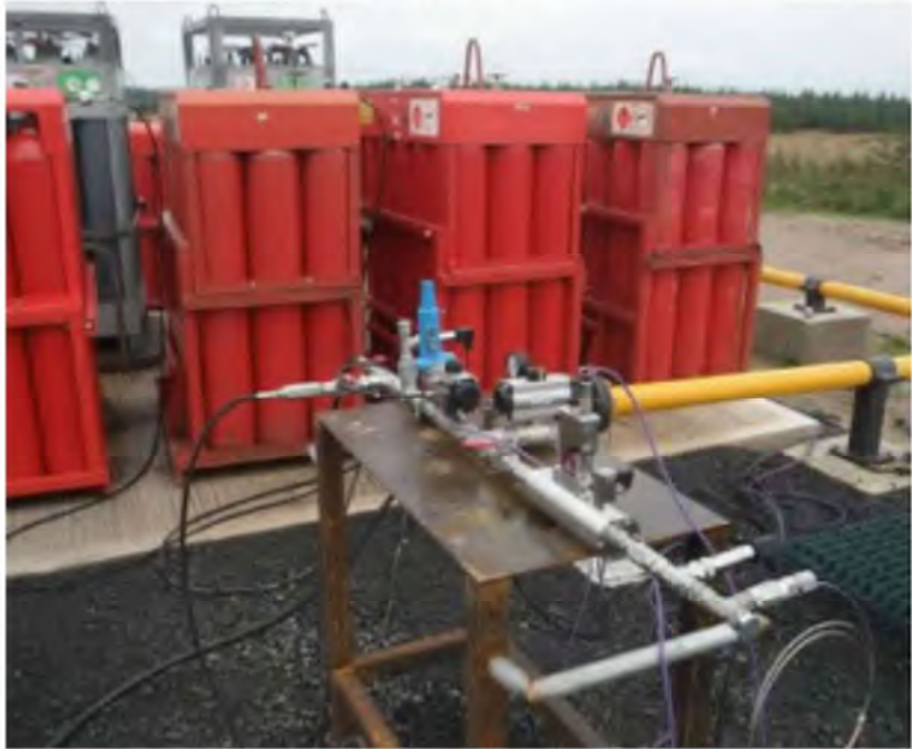
Figure 17: Release control arrangement
