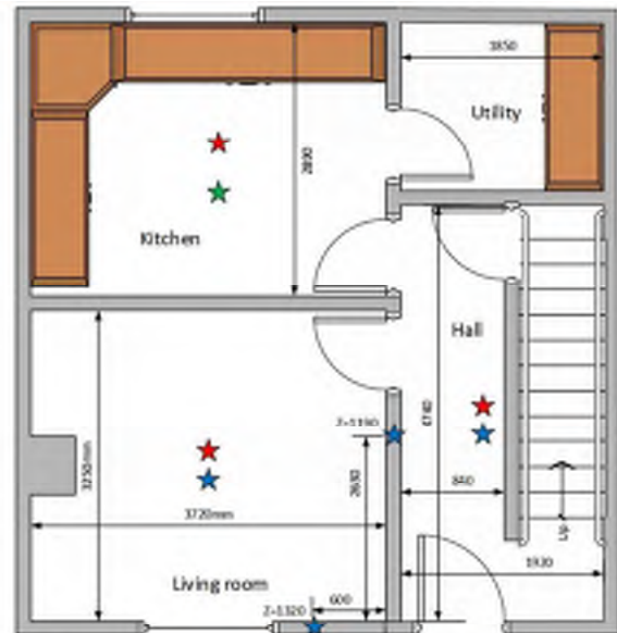
Figure 21: Ground floor sample point locations for basement releases
