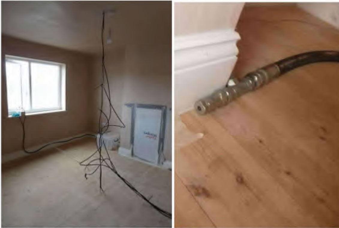
Figure 5: Living room and release point (shown with enhanced sample line arrangement used in Phase 2 (L3-A19 and L3-A20))
