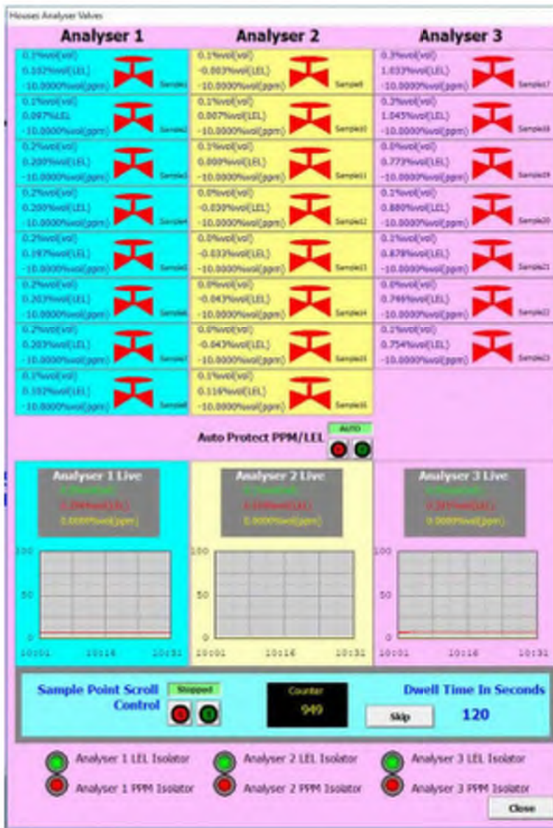
Figure 31: Hy Street SCADA screen for sample point monitoring and last known values.
