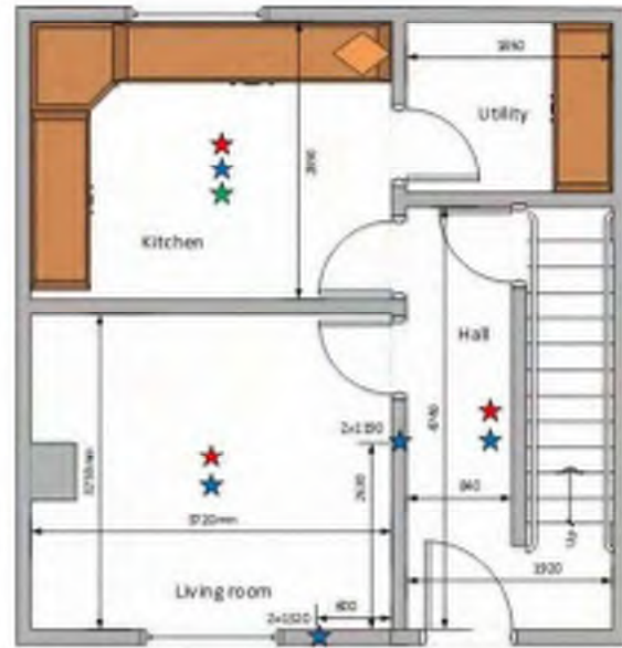
Figure 23: Ground floor sample point locations for kitchen boiler cupboard releases
