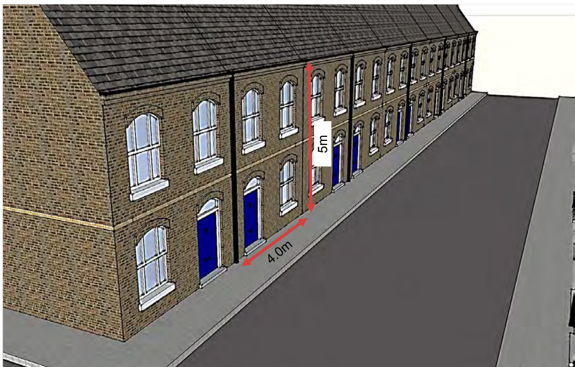
Figure 22: Some estimated dimensions used to model a residential property in a typical setting (Extract of Sketchup image from [20])
