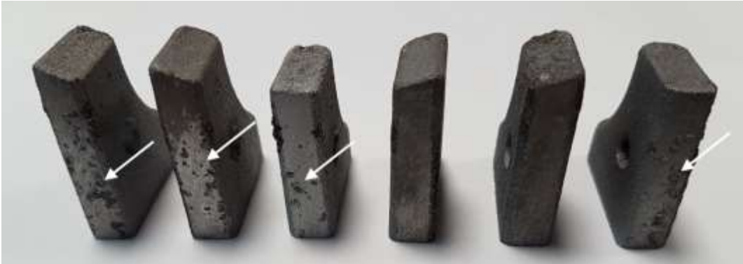
Figure 12: Photograph of WB6 specimens tested in condensate A to E (left to right), showing preferential pitting corrosion of the machined face.
