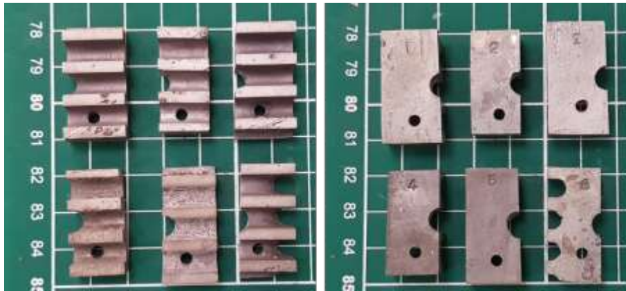
Figure 8: Post-test images of the WB7 specimens tested in condensate A to F (left to right, top to bottom).
