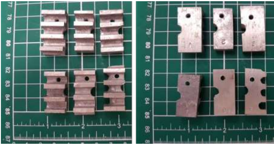
Figure 5: Pre-test images of the WB7 specimens tested in condensate A to F (left to right, top to bottom).
