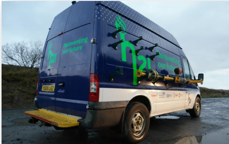
NGN vehicle fitted with metering and detection equipment required to ensure the accuracy of the Hydrogen injection
